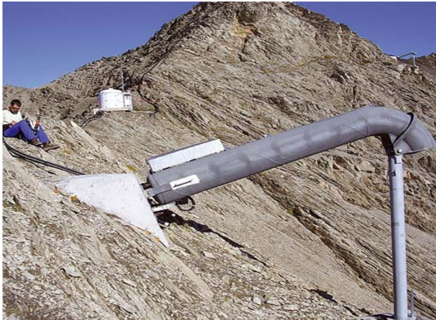
Figure 4. Technologie Alpine de Securite' (TAS) fixed, remotely operable avalanche initiating gas blaster.
