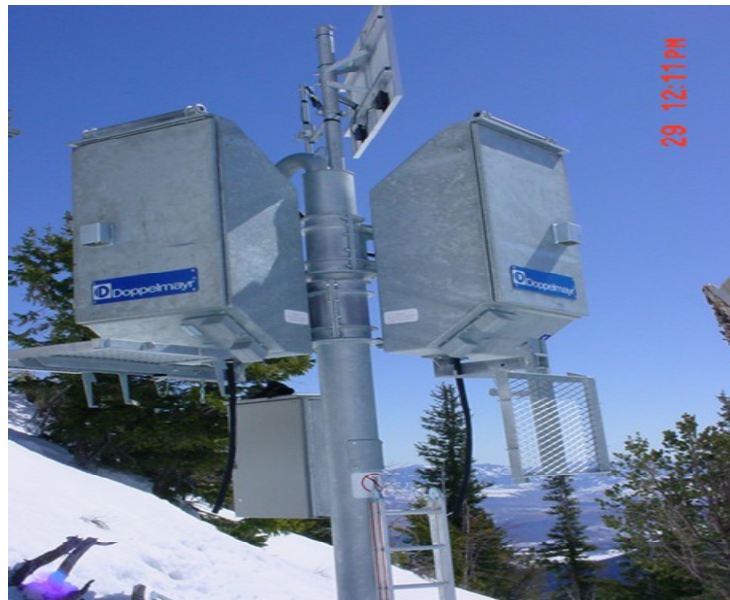
Figure 3. A remotely operable avalanche control "mortar" in the starting zone of an avalanche that threatens the roadway below.
